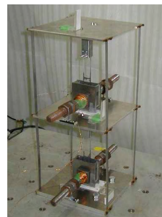
Fig. 6 2DOF model with MR damper
